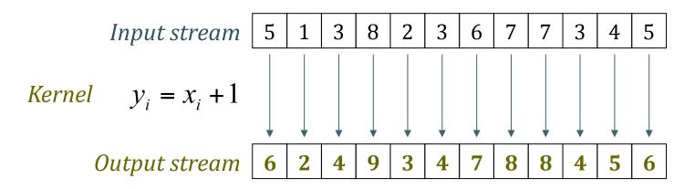
• GPUs excel at this thanks to a large number of processing units and a parallel architecture
