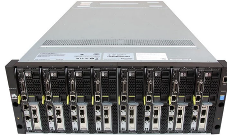
Figure 2: Computer (node) from the Graham super computer.
